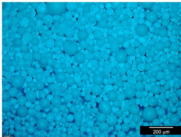
**Fig. 5 – Optical micrograph of spray-dried 3Y-TZP powder particulates.**
